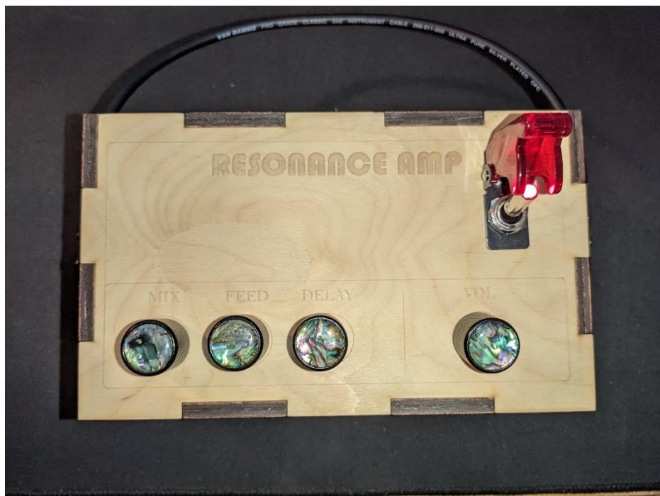
Figure 19: Top down of unit turned on with LED power indicator switch.
