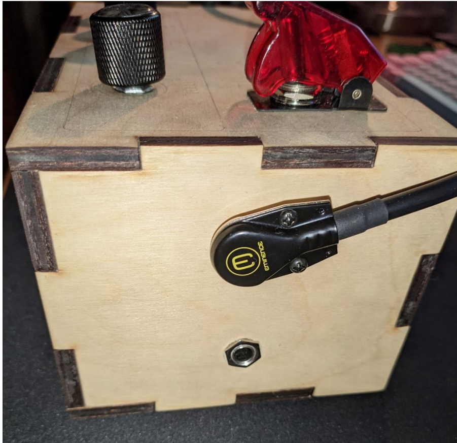
Figure 22: Left side view showing effects loop out (top) and stereo input/output (bottom)
