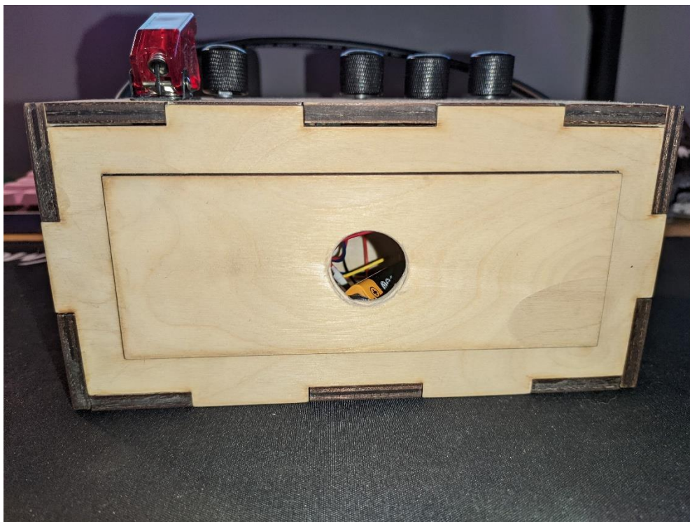
Figure 20: Back view showing removable back panel with finger pull / external power route.
