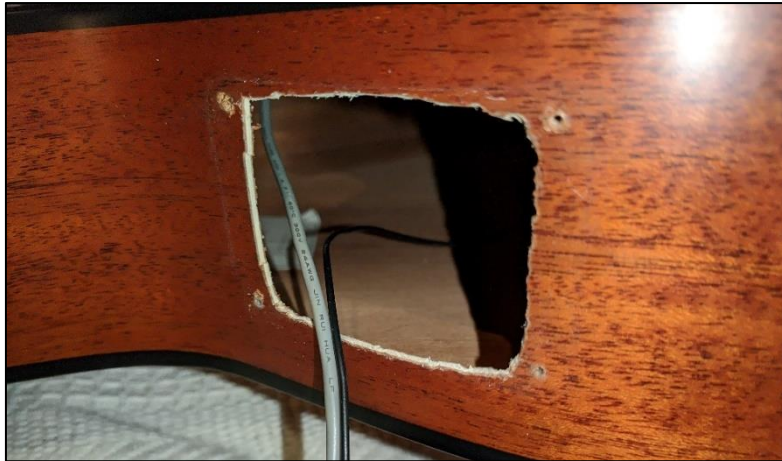
Figure 25: Mounting hole for pre-amp circuit.
