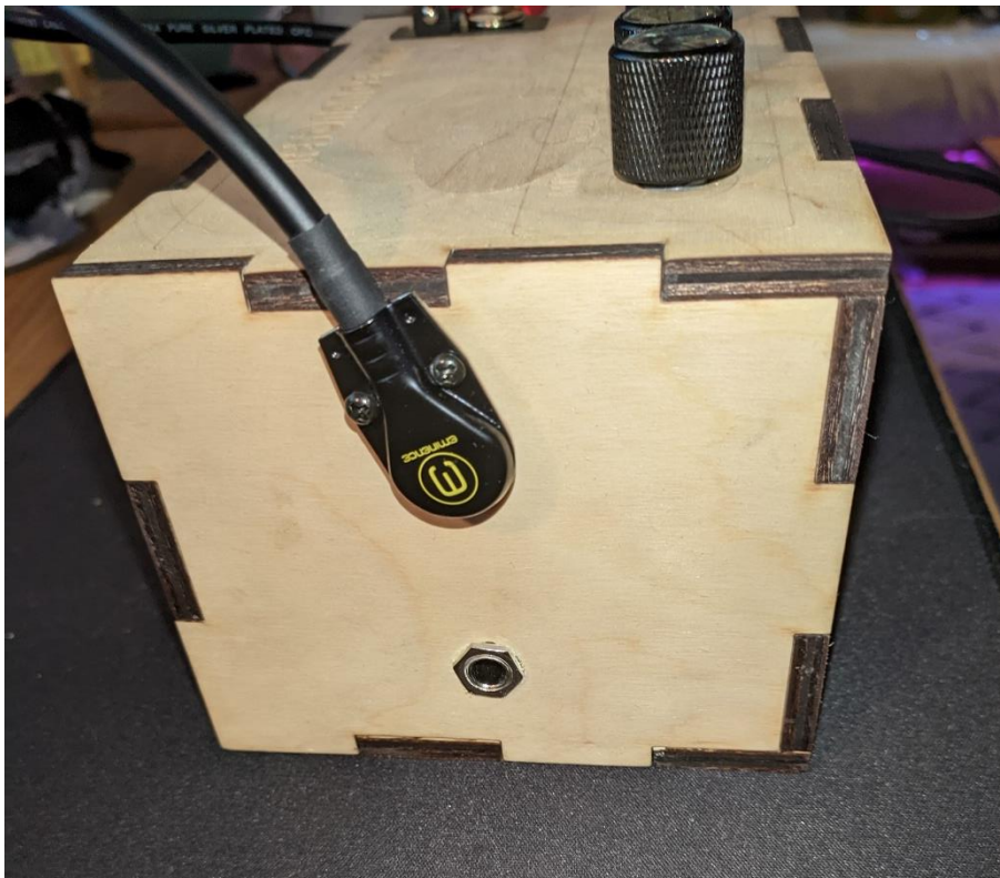
Figure 23: Right side view showing effects loop in / mono input (top) and external speaker output (bottom)
