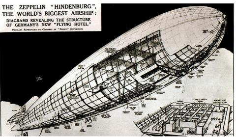
Fig. 33 Hindenburg interior structure diagram
