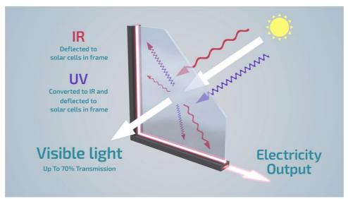
Fig. 24 Diagram of ClearVUE Solar Glass, ClearVUE Source
