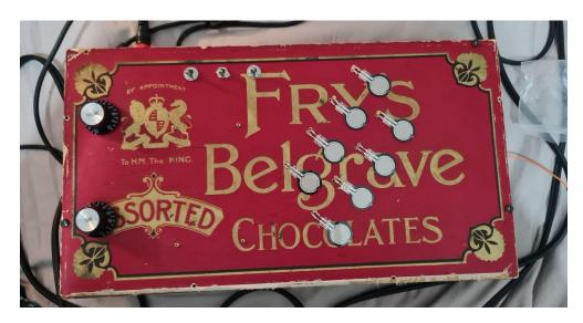
c.3, Circuit for force sensitive resistors
