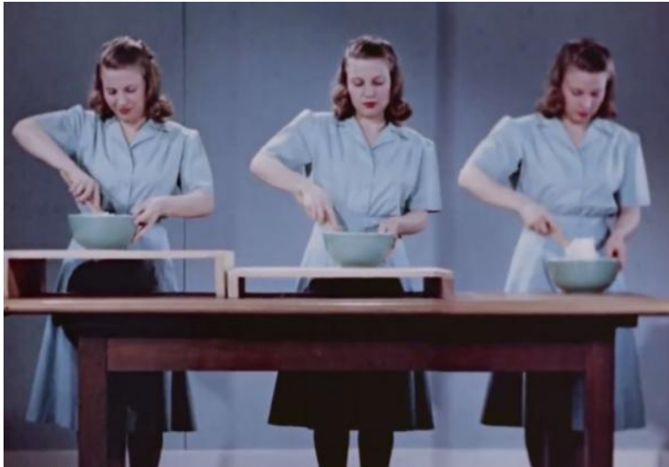
Figure 10 Testing of different working surface heights per task. Visual from National Agricultural Library. U.S. DEPARTMENT OF AGRICULTURE “Step-Saving Kitchens”. Accessed on 04 Oct 2023. Web.
