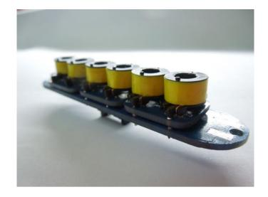
Figure 54 showed the fully assembled Hexophonic pickup (Guzman, 2013)
