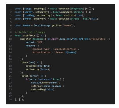
Figure 43 illustrated the useFetch that request to the API for the list of songs.
