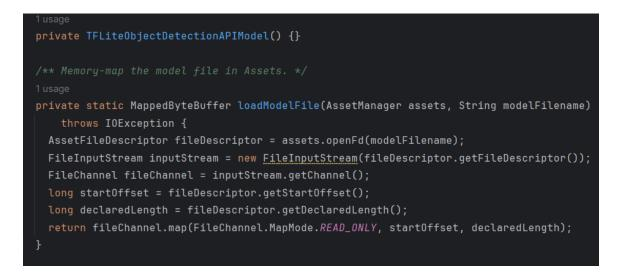
Figure 5.3.4 – Loading a TensorFlow Lite model
