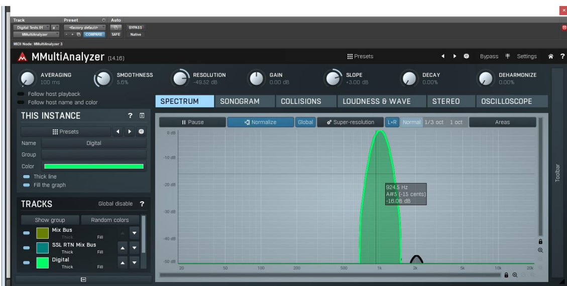
Appendix Figure 1.7 Second Harmonic on Analog Distressor
