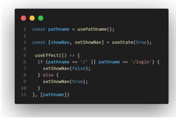
Figure 67 Logic to show the bottom navbar on specific routes
