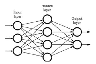
Figure 2.3 How a simple Neural Network works.
